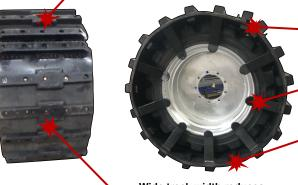
Wide track width reduces ground pressure improve machine stability
