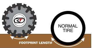
Reduced track depth requires less power with more traction and less soil compaction Increased Footprint Length uses more power, increasing fuel consumption and cause rutting damage
