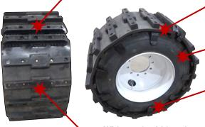
Wide track width reduces ground pressure and rolling resistence
