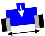
Wide tracks lower the center of gravity and privides better stability on side hill applications
