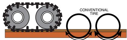
Increase foot print lets machine float over soft ground reducing rolling resistance and drag
